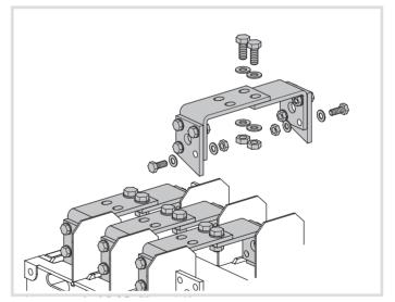
It is possible to mount the bridging bars on either side of the switch.
