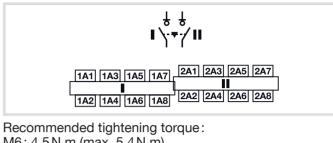
Recommended tightening torque M6: 4,5N.m (max. 5,4N.m) M8: 8,3N.m (max. 13N.m) M10: 20N.m (max. 26N.m) M12: 40N.m (max. 45N.m)
